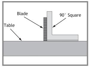
Figure 88. Checking the blade at 90°.
